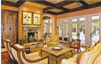
The living room has a Scottish stone fireplace, 120-year-old Balines Palace antique doors, cedar beams from Vancouver, British Columbia, and Venetian plaster ceilings.
